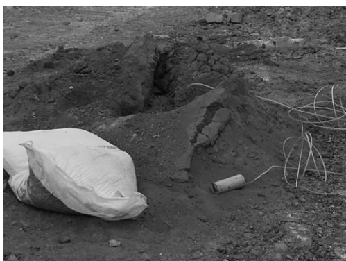
Figure 4. Example of priming bad practices (left) and hole length deviation (right)
