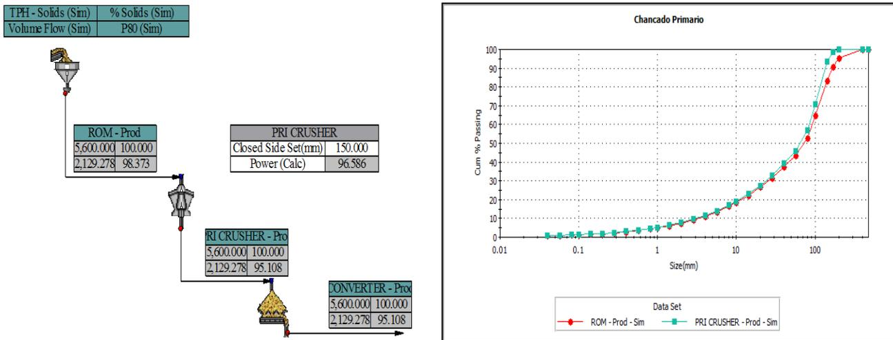
Figure 3. Simulation of primary crushing using SED-H rock type with powder factor of 0.44 kg/t.
