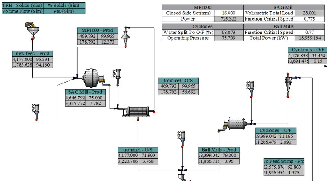
Figure 4. Simulation of grinding circuit using SED-H rock type with powder factor of 0.44 kg/t.
