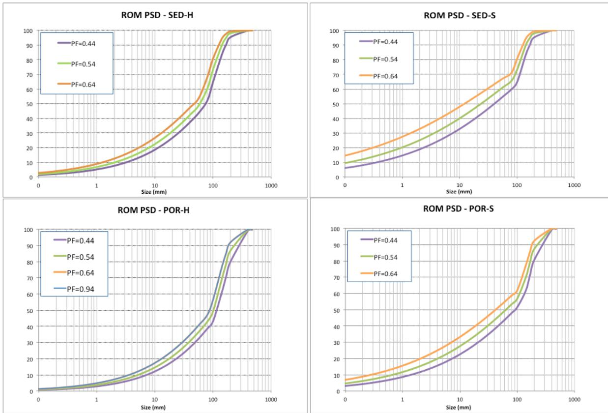
**Figure 2. Run-of-mine particle size distributions for the four geologic units (SED-H, SED-S, POR-H, POR-S) and for the four blast design case studies (0.44, 0.54, 0.65, 0.94 powder factors). The 0.94 powder factor only used for POR-H.**
