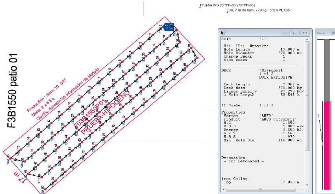
Figure 1. Example of fragmentation analysis using JKSimBlast software.
