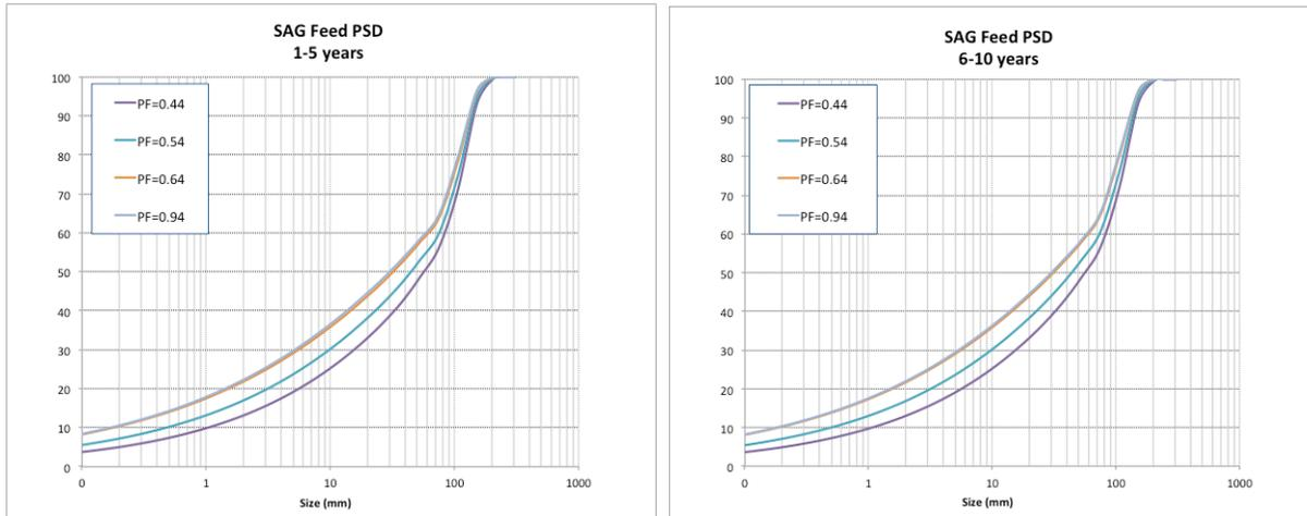
**Figure 5. SAG feed particle size distributions for rock mined 1-5 years and 6-10 years**
